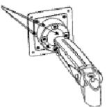
b) Vertical Movement. Adjusting might be required. Use the wrench provided in the accessory kit. If the arm tends to drift down or rise up when positioned, it will be necessary to make a small adjustment in the adjustment screw (see graphic bellow).
