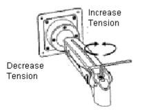
Note: To prevent damage to the arm, remove the wrench before releasing the arm from the horizontal adjustment position.
